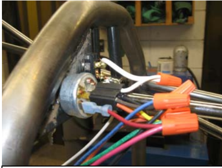
Wiring to ignition and kill switch
